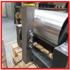
2.22Ø12mm shaft are welded on the stand
