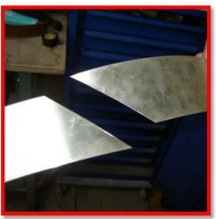
2.6 Lightly smooth skive joint with fine file to eliminate any roughness
