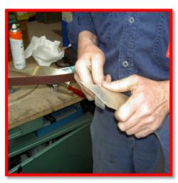
2.7 Spray presavation oil on the shaft See datasheet. (BAC does not supply this)
