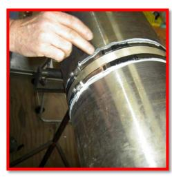
2.15Wrap sensitive tape on one of the steel bands to make it absolutely tight
