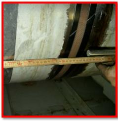
2.2 Sand the area on the shaft between the two straps, until a bright steel surface appears.
