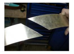
Lightly smooth skive joint with fine file to eliminate any roughness
