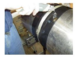
The finish mounting of the shaft grounding before finishing the silver band
