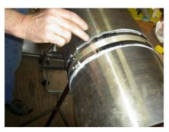
Wrap sensitive tape on one of the steel bands to make it absolutely tight
